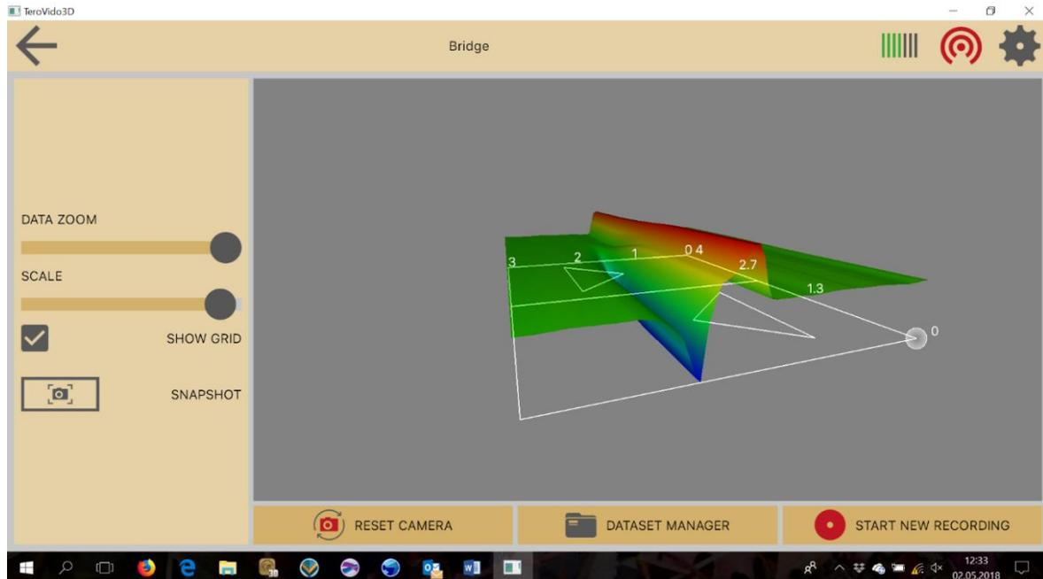
After recording this window opens. Here you find the value analysis with different settings. On the one hand you can change the data zoom and the scaling. Furthermore you can show or hide the grid.
